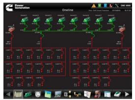
The one-line diagram screen displays system status by a combination of animation, changing screen color, text messages, and pop-up indicators. Conditions visible on the screen include:
