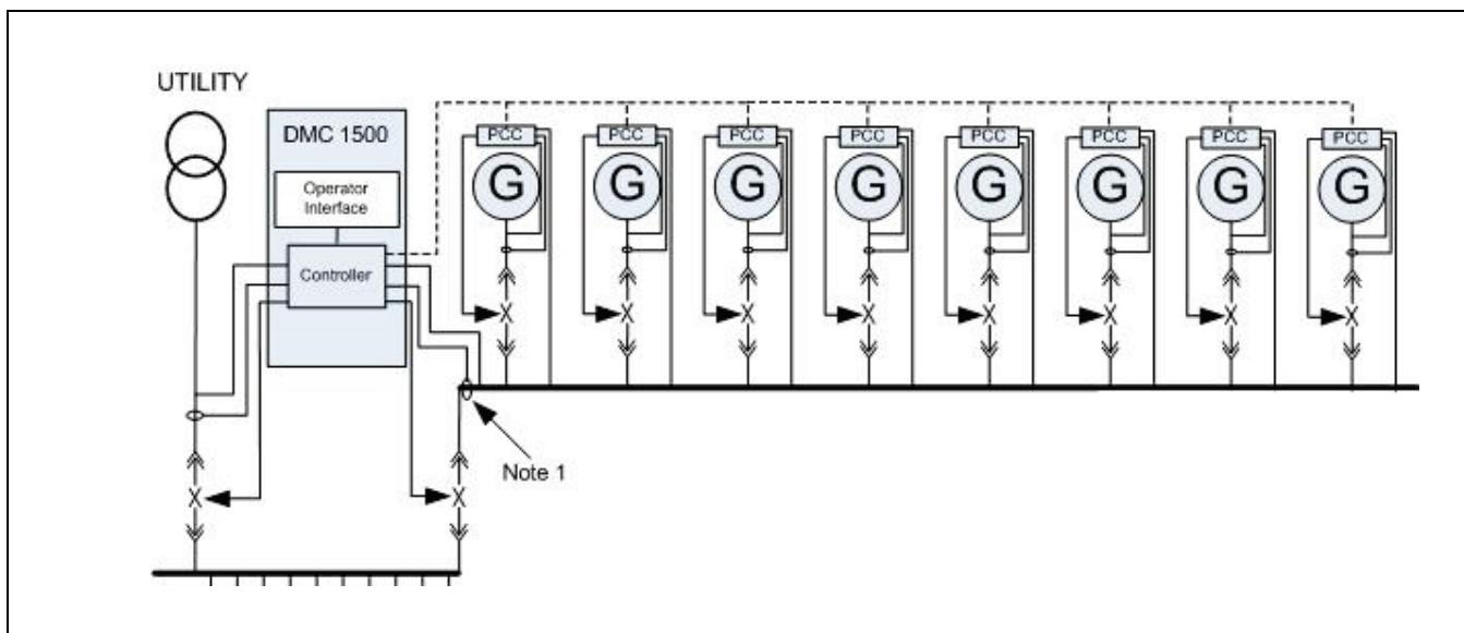
**NOTE 1:** Current transformer (CT) sizing and location must be considered as part of the design and physical layout of the power section. The generator bus CT connection presented in the one-line diagrams above represents totalized generator bus current output.
