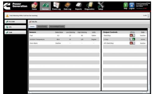
Clicking on the Home Page building icon navigates the user to the details page, providing a snapshot of all configured sensors or output controls.
